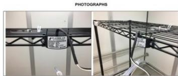
Left: Air cleaner placement in chamber for testing
